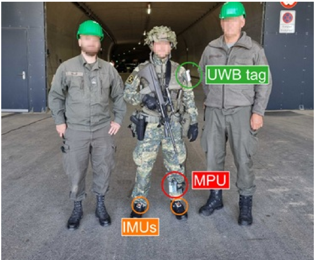
► Military troops equipped with the NIKE BLUETRACK system at the demonstration event IRON NIKE. [Source: IfG der TU Graz]
