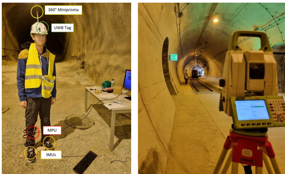
Figure 3: Test subject with sensors mounted on helmet and shoes (left). ERT with Leica MultiStation used as reference in front (right)
