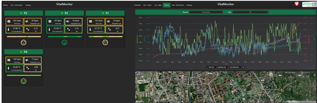
Figure 3: Examples of VitalMonitor real-time visualisation of vital parameters, thresholds, stress index and location.
