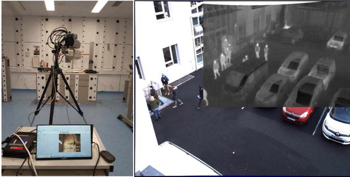
Figure 2: Geometric calibration of the S-RGBT camera system in the measurement lab (IGMS/TUG); Synchronized and co-registered image sample where parts of the TIR image are superimposed on the RGB image.
