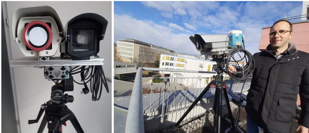
Figure 1: Combined RGB/TIR camera prototype mounted on a tripod, first test recordings at JR DIGITAL, Steyrergasse 17, Graz (4 th floor).
