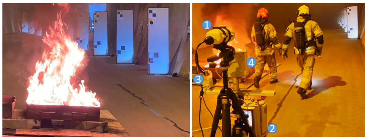
Figure 4: Fire cup and sensor setup: 1-Video camera, 2-Terrestrial laser scanner, 3-Thermal camera, 4-RADAR sensor.
