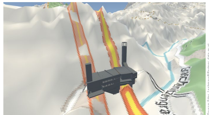
Fig. 5 BIM-model, portal building Karawankentunnel, visualized in SOMT.
