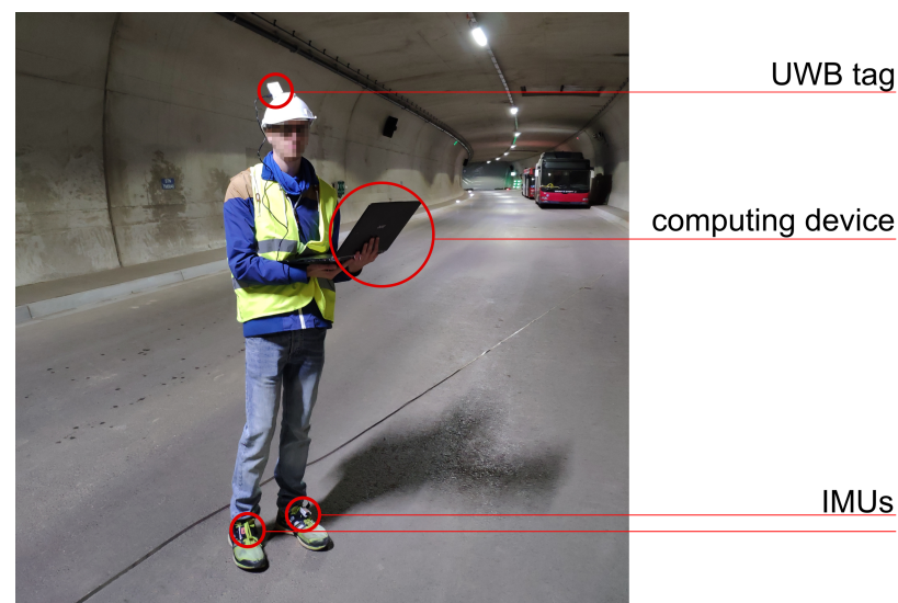
Figure 11. Test subject with sensors mounted on helmet and shoes.
