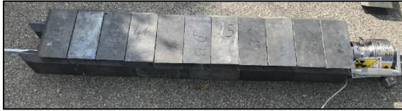
Illustration 2: Small Scale Straight Tunnel Made with Lead Shielding Bricks
