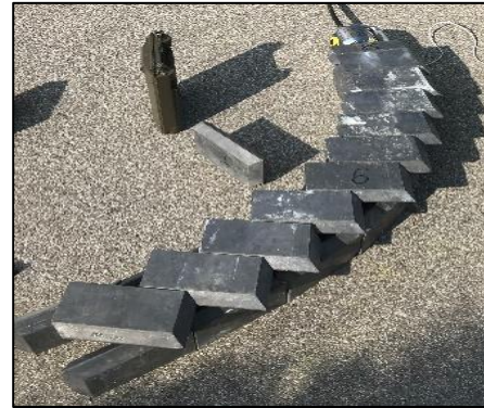
Illustration 4: Small Scale Curved Tunnel Made with Lead Shielding Bricks
