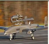
The pulsejet-powered Scitor-D reflects growing interest in low-cost, high-performance engines for decoys, one-way attack drones, and more.
