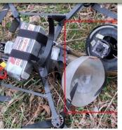
Russian forces in Ukraine appear to now be using FPV kamikaze drones controlled via a physical fiber optic line rather than a wireless data link. This configuration offers a control method that is immune to radiofrequency electronic warfare, but that also imposes certain limitations...
