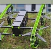
A consortium of 7 partners from the EU has successfully completed the concept of a hybrid UAV-UGV drone. It combines the most useful and necessary features of a flying drone with a riding drone.
