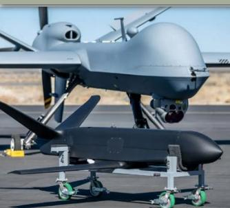
A2LE is a new drone from General Atomics that leverages rapid design and manufacturing that could pave the way to future air-launched swarms.
