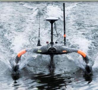
Sonobot 5 is mainly used for three-dimensional mapping. The device can be used during search operations to identify objects that pose a threat to the safety of people and infrastructure.
