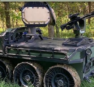
With a smart gunsight, rifle, radar aboard a small uncrewed ground vehicle, a new counter-drone system can follow troops where they go.
