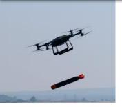
The T-600 is an electric-powered demonstrator aircraft capable of vertical take-off and landing, can carry a payload of 200kg and can travel at up to 140km/h.
