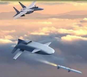
The LongShot program is centered on developing an air-to-air missile-armed drone that fighters and bombers can launch and control.
