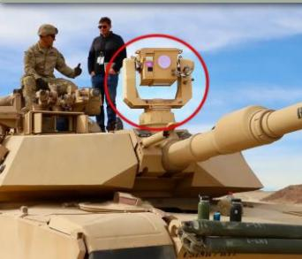
The Advanced Targeting and Lethality Aided System provides tank operators with computer-generated target and fire options.
