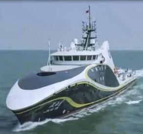
It can carry and operate dozens of unmanned aerial, surface and underwater vehicles (UAVs, USVs and UUVs) simultaneously to monitor its surroundings and produce a data hub.
