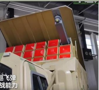
The highly-mobile truck-mounted swarm launcher can hold 18 drones that can execute strike, surveillance, and possibly other functions.
