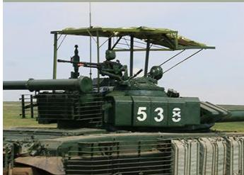
Screens to defend against top-attack weapons have been seen fitted to Russian Airborne Forces (VDV) T-72 tanks during an exercise in Crimea.
